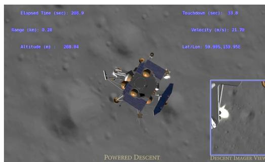
**Figure 2. ETV for MoonRise Lunar Sample return proposal.** ETV can visualize simulated spacecraft-acquired imagery using actual camera pointing and field of view information.
