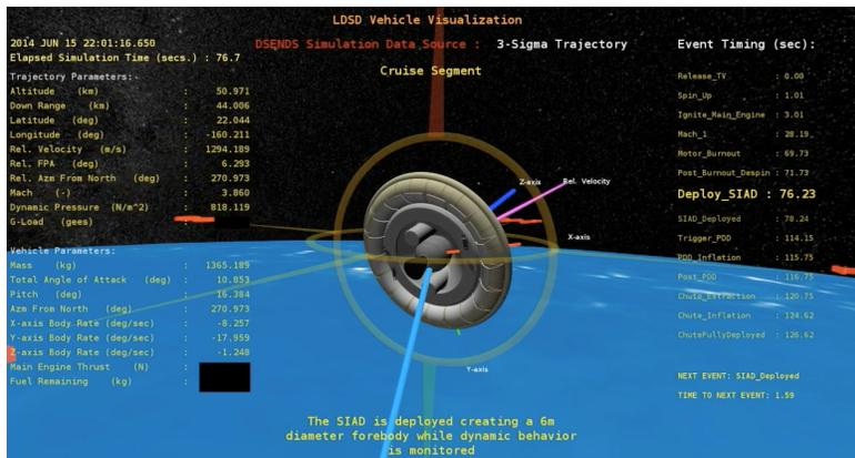
**Figure 4. ETV Supporting LDSO Flight Simulation.** ETV receives mission telemetry data and displays vehicle state and health using polygon-based 3D spacecraft and environment representations, as well as run-time updated tabular data and ornamental CAD items such as compass araphics, velocity and line-of-siaht vectors.
