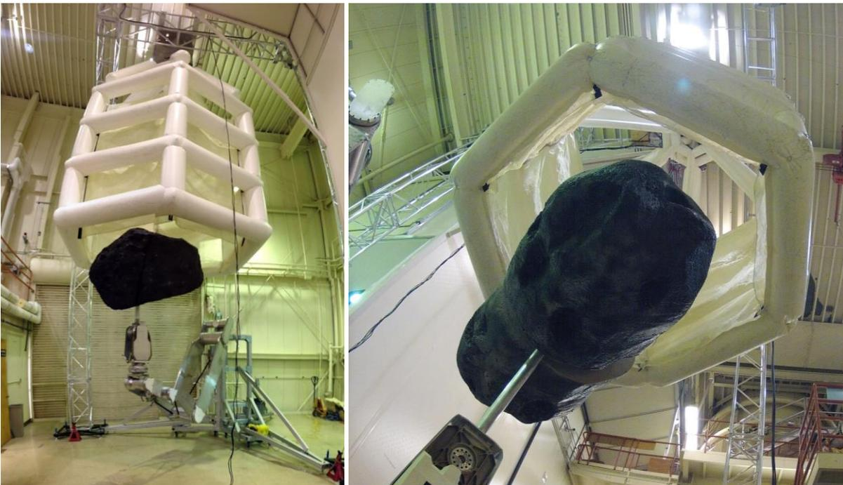
Figure 3: Early feasibility capture study using inflatable testbed
