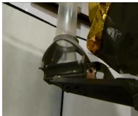
Figure 14: Detail of pinch-roller winch on Option A capture testbed
