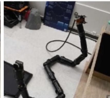
**Figure 18 Non-mobility behaviors of EELS. Left: "head up" behavior for increasing the range of onboard perception. Right: Manipulation behavior with a gripper at the tail section.**
