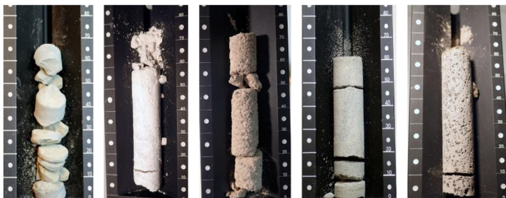
**Figure 2. Examples of rock cores of the five rock types collected in the Qualification Model Dirty Testing.** The tests of the coring drill were performed only on six geo-analog rock types, which were later downselected to five. From left to right: Kramer Massive Mudstone (KMM), China Ranch Gypsum (CRG), Bishop Tuff Intermediate (BTI), Napa Basaltic Sandstone (NBS), and Uniform Saddleback Basalt (USB). Image from (Moeller, et al. 2021). Credit: NASA/JPL-Caltech.
