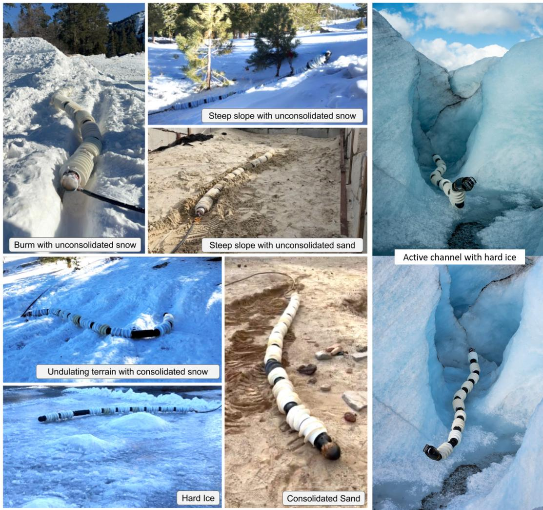
**Figure 6** The EELS 1.0 robot traversing over mobility-stressing extreme terrains
