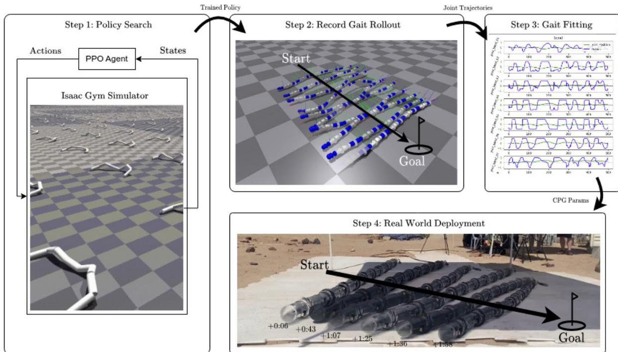
**Figure 8 Process for training robust reinforcement learning policies and converting them to hybrid control approaches [11]**
