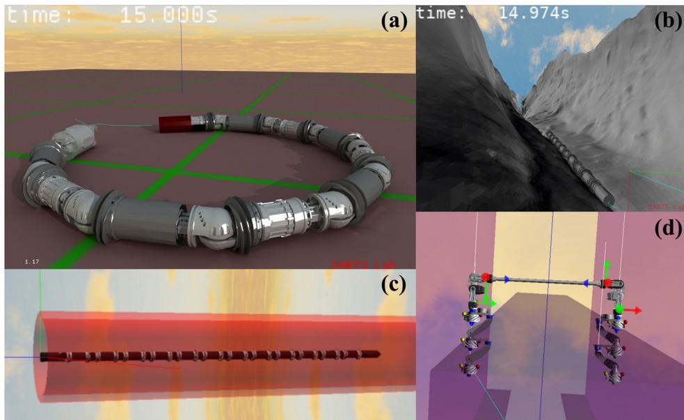
**Figure 12** Different terrains within the DARTS environment, with EELS 1.0 and EELS 1.5 models being tested [16]
