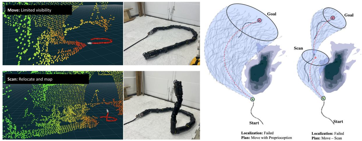
**Figure 10** NEO's Risk-aware Integrated Task and Motion Planning Framework in a Moulin Avoidance Mission Scenario. Joint reasoning about moving and scanning activities along with risk-awareness allows the robot to come up with more optimal paths while satisfying safety constraints.
