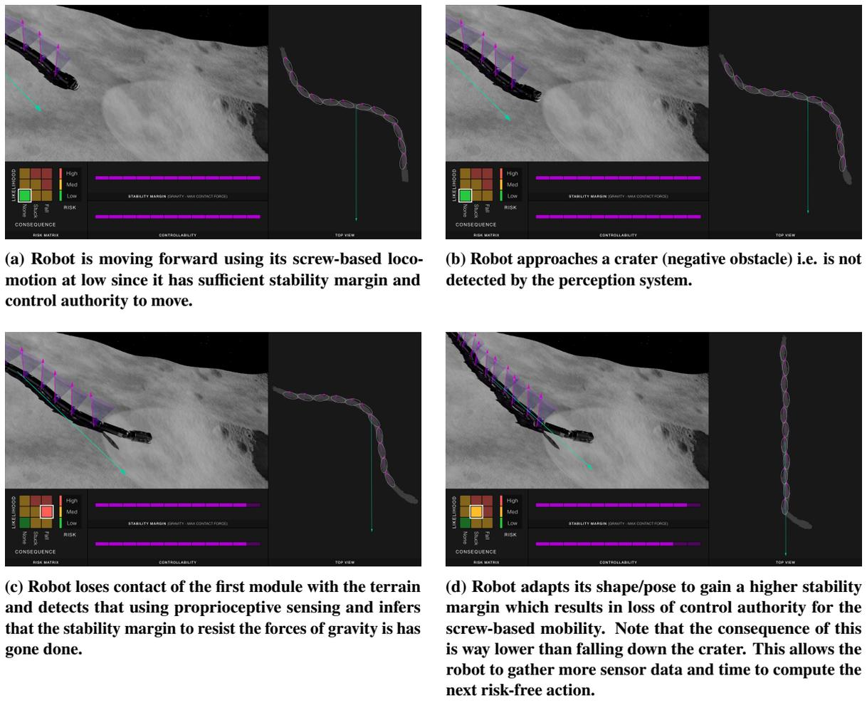
**Figure 9** NEO's On-board Risk Matrix-based Adaptation in a Lunar Crater Navigation Mission Scenario.
