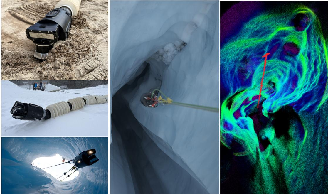
(a) EELS 1.0 sensor head deployed in extreme environments (b) 3-D reconstruction of a Moulin at Athabasca Glacier using NEO's SLAM algorithm, SERPENT [4].
