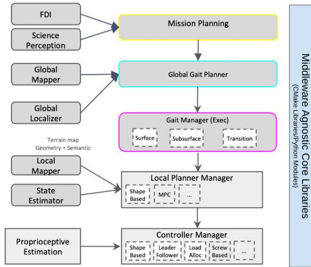
**Figure 13** Software Architecture to enable Agile Autonomy Development by implementing core capabilities as middleware-agnostic core libraries.
