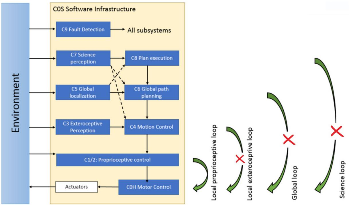
Figure 3 Module architecture for NEO, displaying the resilience provided by the framework; when higher level modules fail, the mission continues
