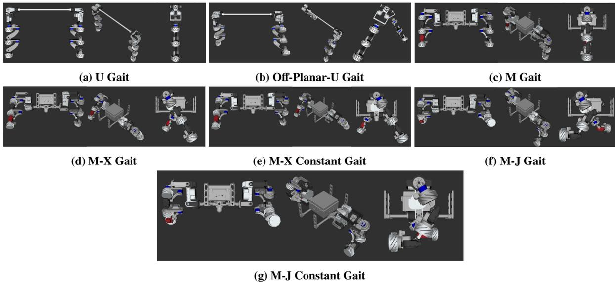
**Figure 14** Gaits iterated through during the development of the EELS 1.5 platform [7] (For each image: Left: Front View; Center: Isometric View; Right: Side View)
