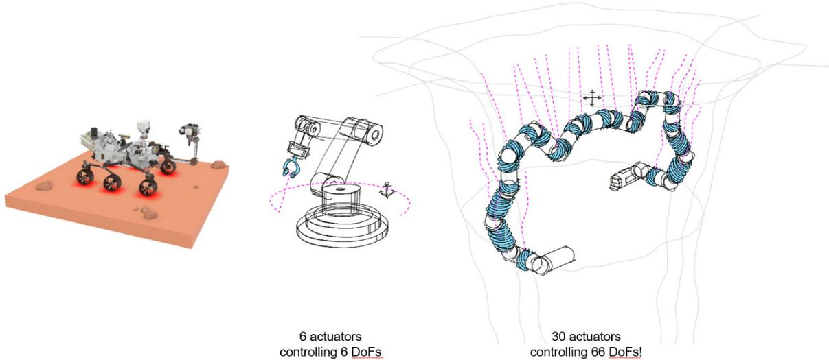
**Figure 5 EELS as a Loco-manipulator: The Perseverance Mars Rover, a generic manipulator, and an EELS concept robot juxtaposed together**
