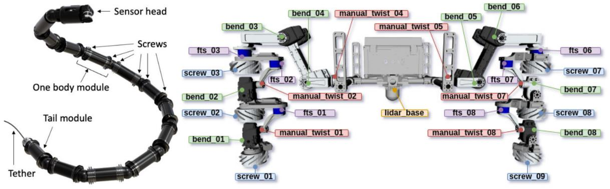
Figure 2 The EELS 1.0 and EELS 1.5 platforms, respectively
